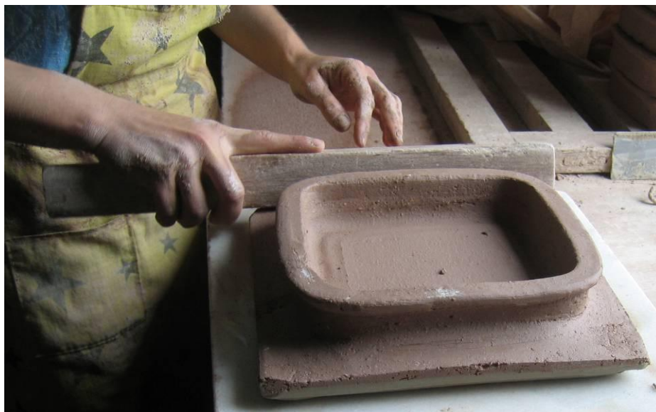
Fig. 1.21. Attaching the back rim to a panel tile. 57
