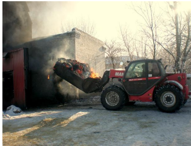
Figure 2-4. A tractor with front-end loader used to feed in straw bales to the boiler and remove bottom ash (Photo: Courtesy of V. Belay)
