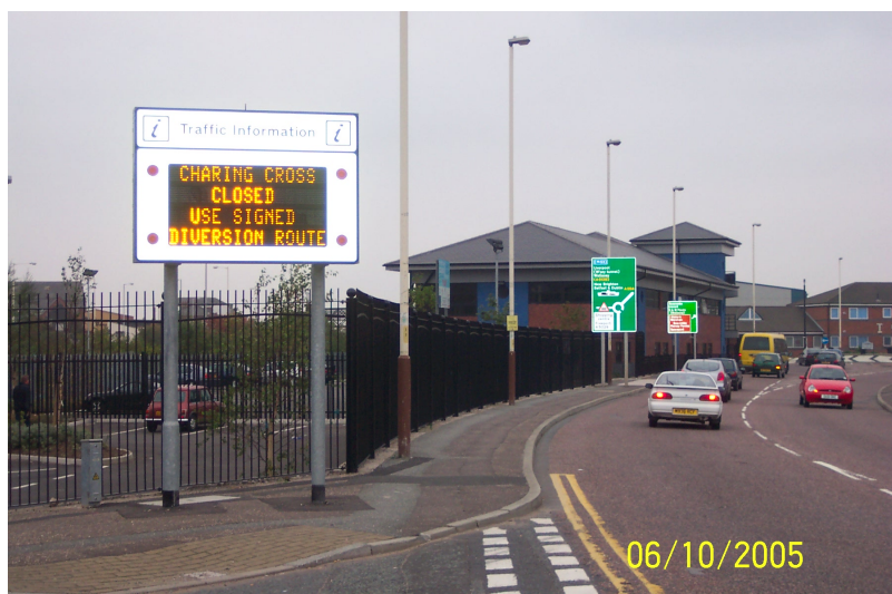
Figure I:2 “Variable Message Sign” to advise drivers on traffic changes, Wirral, Mersey, UK
