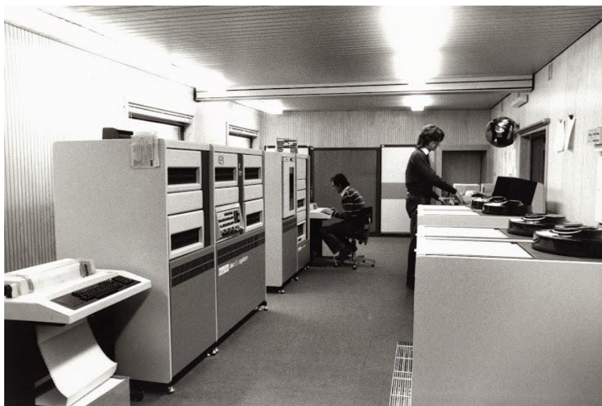
Fig. 2.2. This picture shows the data processing center at RFE-Munich in the 1970s when the radio technical team installed a new computer for data analyses. The machine was Digital Equipment, model PDP-11, which replaced the older models (with IBM punch cards) used until the 1960s when the radio relied mainly on external institutions for processing large amounts of data.
