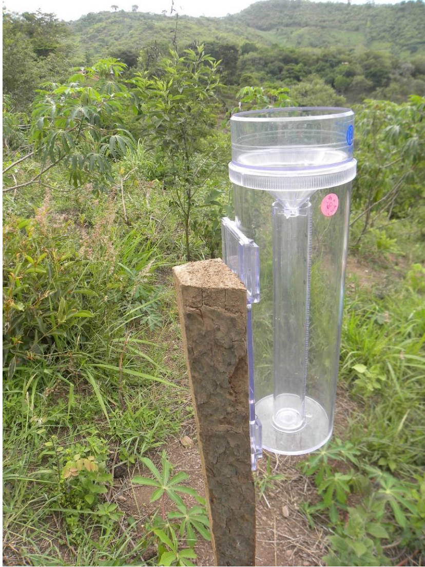
Picture 10. Rain gauge or pluviometer installed by a climate change adaptation project in El Nancite
