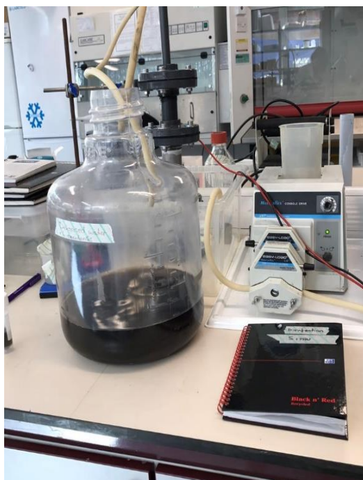
Fig 3.3 The black effluent after 48-hour treatment at 0.5A current intensity.
