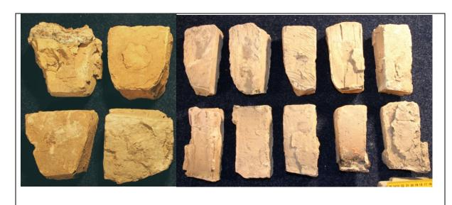
FIG. 71. Characteristic building blocks of glass furnaces
