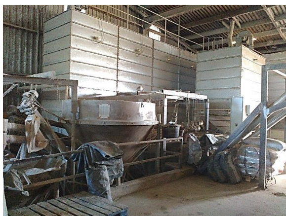
Photograph 44 & Photograph 45. Feeding machinery in conventional and alternative operations A conventional farm feed grinder (left) and alternative farm pelleting apparatus (right) illustrate the differences between the scales of the farms. Note both machines were in operation (source: the author).
