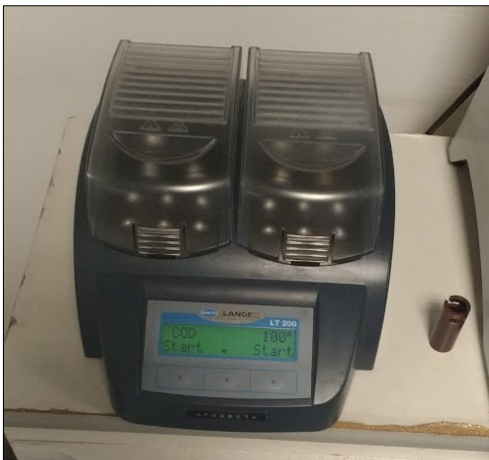
Figure 28: HACH LT200 Thermostat used for the experiment in the laboratory
