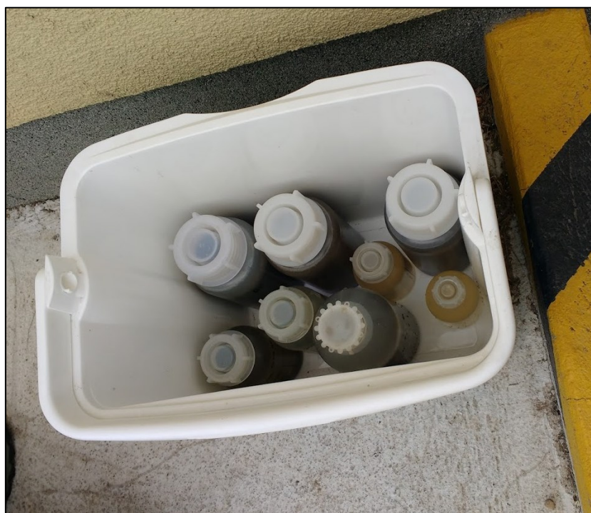
Figure 27: Samples are kept in the cooler box to prevent biological activity
