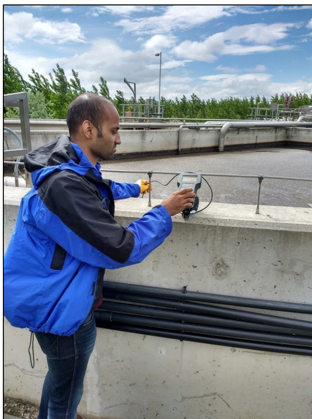
Figure 26: Measuring the sludge concentration using the digital meter
