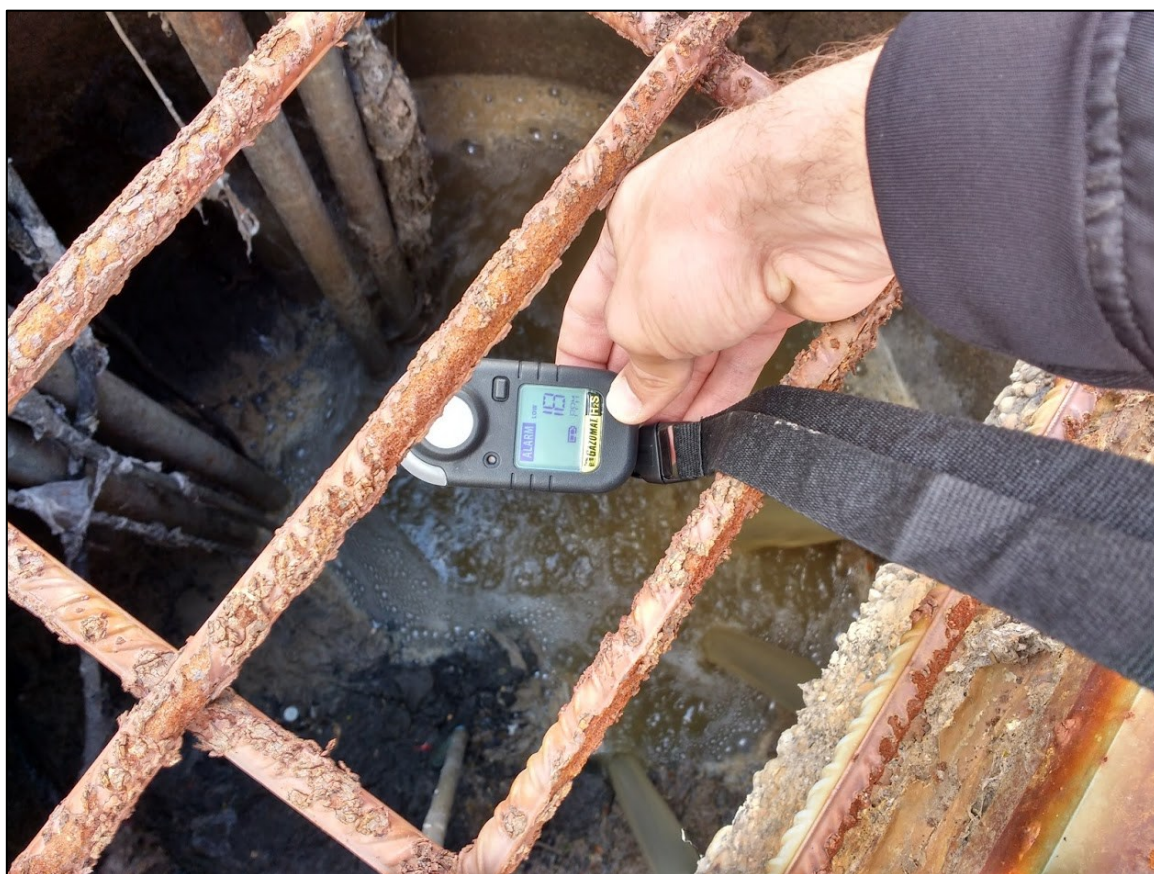
Figure 23: Measuring the ambient concentration of H_2S in the primary tank
