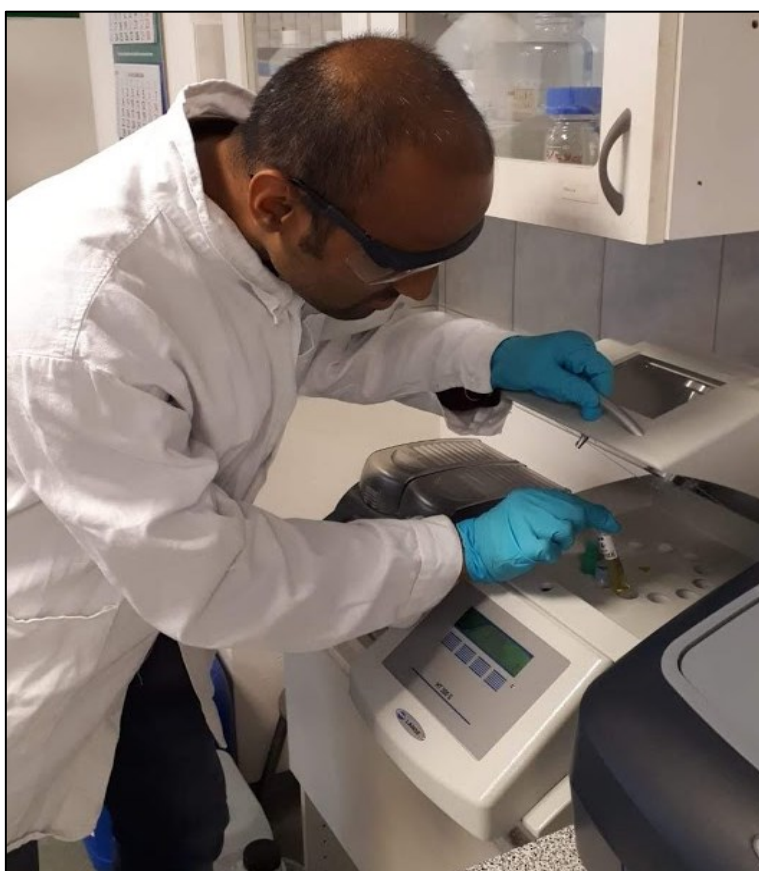
Figure 39: Placing the cuvettes inside the thermostat for heating
