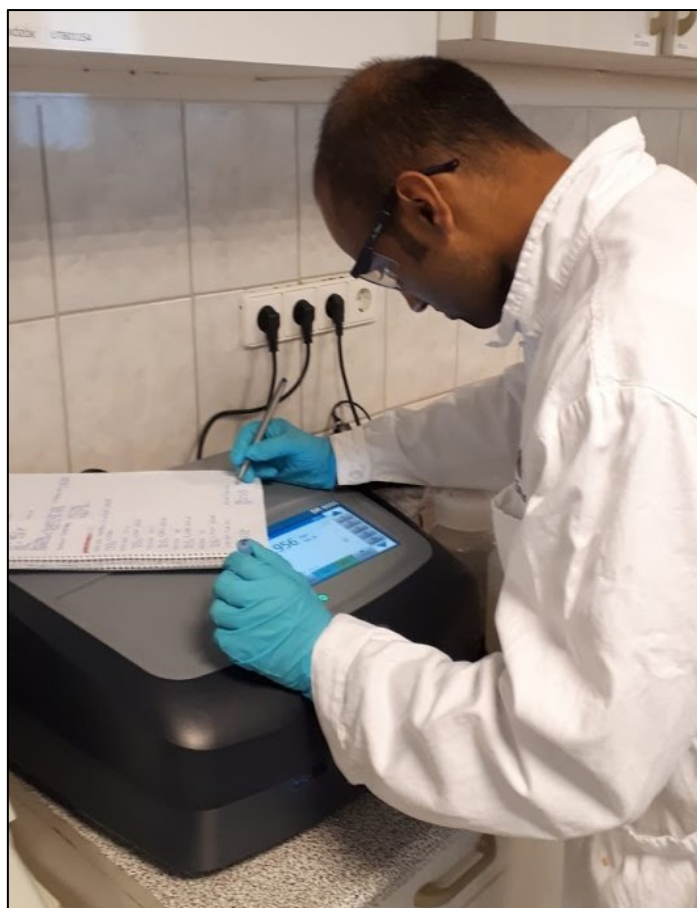
Figure 40: Placing the cuvettes in the photometer and noting down the result
