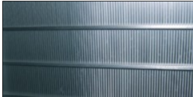
Figure 3: Fine screen (Source: Huber Technology)
