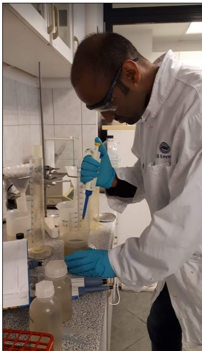
Figure 35: Pipetting 0.2mL of sample cuvette for the testing of \text{NH}_4\text{-N}
