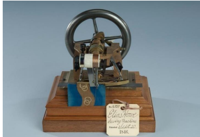
Fig. 43 Elias Howe's sewing machine
