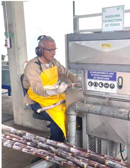
Image 6.3 The machine to extract the yemas (stalks) of sugarcane (left) and the asexual reproduction of stalks in seed beds (right) (own photos).
