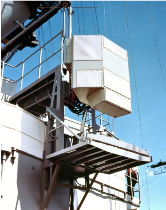
Figure.2.4. The Cold War dialogue on electronic warfare entailed discussions on specific jamming weapons. This is an image of the AN/SLQ-17 electronic warfare system mentioned in a Soviet publication in the 1970s. Photograph 6403938; “A view of the AN/SLQ-17 electronic warfare system aboard the nuclear-powered aircraft carrier USS ENTERPRISE (CVN 65),” January 1, 1978; Records of the Office of the Secretary of Defense, Record Group 330; National Archives at College Park, College Park, MD.
