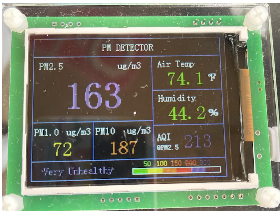
Figure 13. Emission monitor showing the drastic effects smoking has on nearby readings
