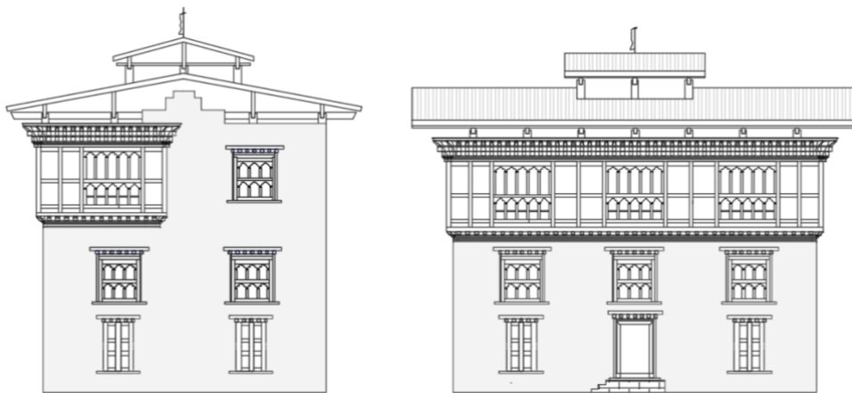
Figure 27. Sub-type 1-three-storied house- Left: side elevation; Right: Front Elevation (Drawing by author)
